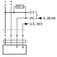
Override control with AC 24 V with Control remotely 0...100% with rotary switch positioner SG..
